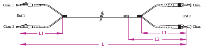
Fig. 3: Flat Duplex Patchcord Schematic
